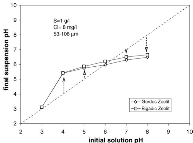
Fig. 3. Change in initial pH after the experiments.
