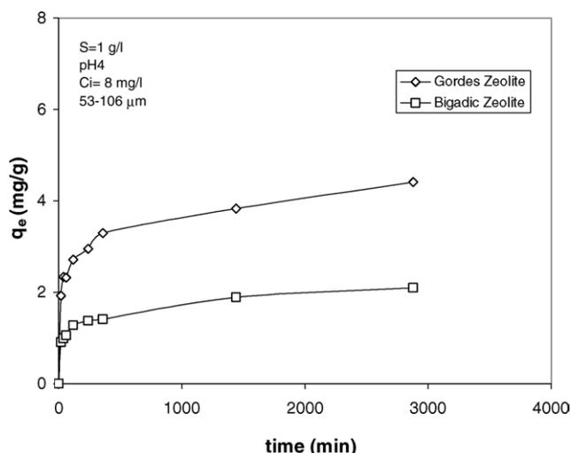
Fig. 1. Adsorption characteristics of materials during 2 days.
