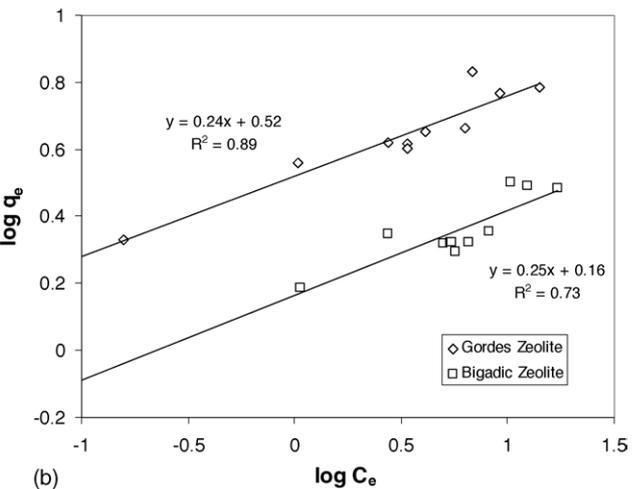
Fig. 6. Linearized (a) Langmuir and (b) Freundlich isotherms for Zn<sup>2+</sup> removal by zeolites.
